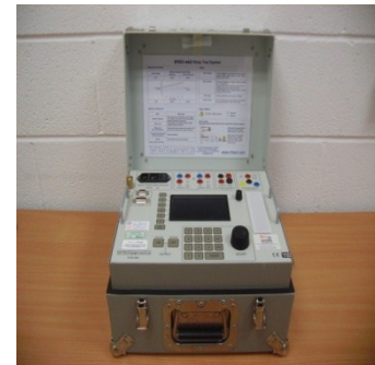
Figure 5 - G59/2 test equipment
