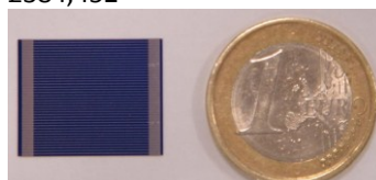
Narec's silicon LGBC 50-sun solar cell (1 Euro coin indicates size)
