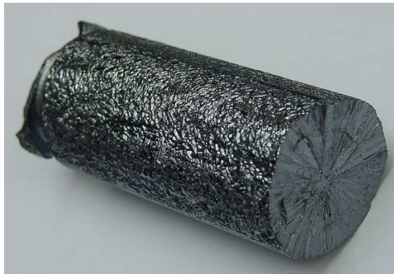
Polycrystalline rod produced by Siemens process
