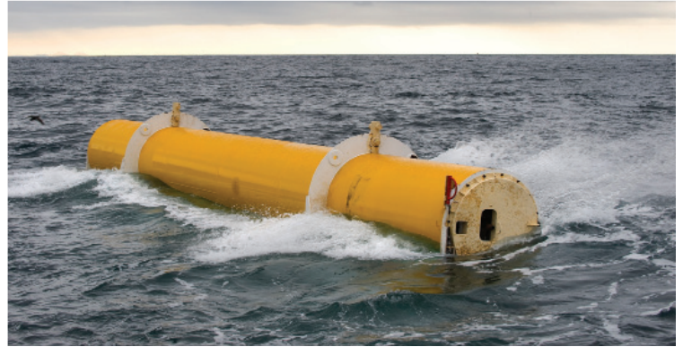
Oyster® Wave Energy Device from Aquamarine Power
