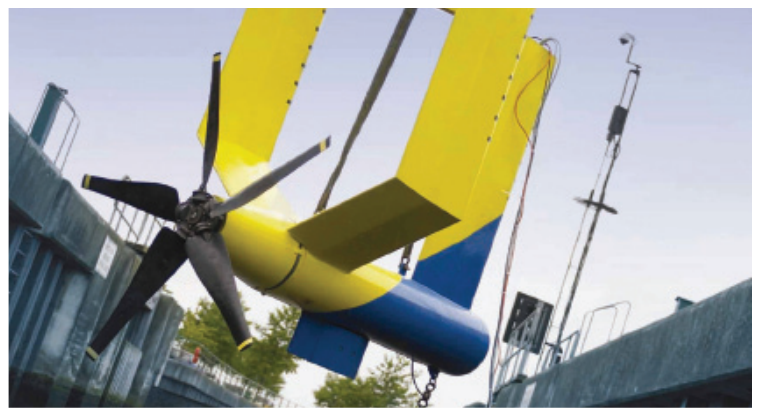
'Evopod' Tidal Turbine from Ocean Flow Energy
