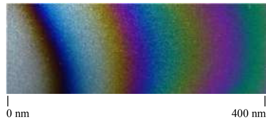
Figure 3: Interference colours in a silicon nitride layer of varying thickness on a non-textured monocrystalline silicon surface
