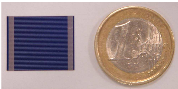
Fig. 2. Left: A two bus bar LGBC silicon concentrator cell designed for 50X, Right: 1 Euro coin for size comparison.
