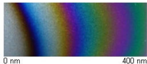
Figure 2: Interference colours in a silicon nitride layer of varying thickness on a non-textured monocrystalline silicon surface
