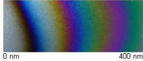
Figure 2: Interference colours in a silicon nitride layer of varying thickness on a non-textured monocrystalline silicon surface
