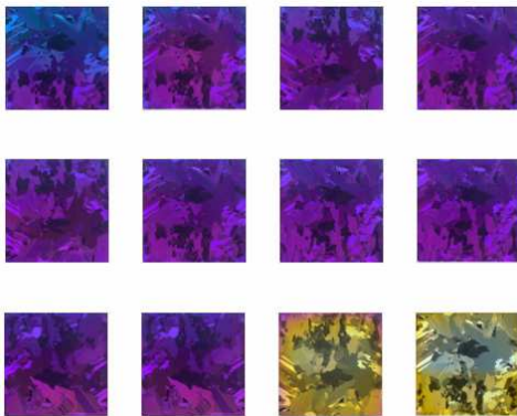
Figure 5: Results of the trial to evaluate uniformity of colour along the LPCVD process tube.
