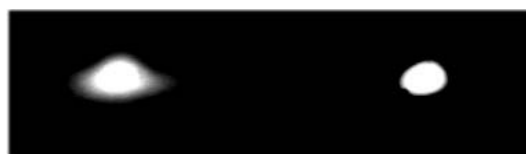
Fig. 9 Measured images of the fundamental modes for rib widths of 4 \mu\text{m}
